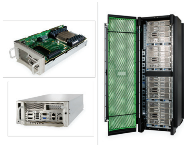
Figure 17: SGI 2000 SMP and Compute and Base I/O blades
