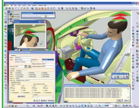
Exit head clearance evaluation.
