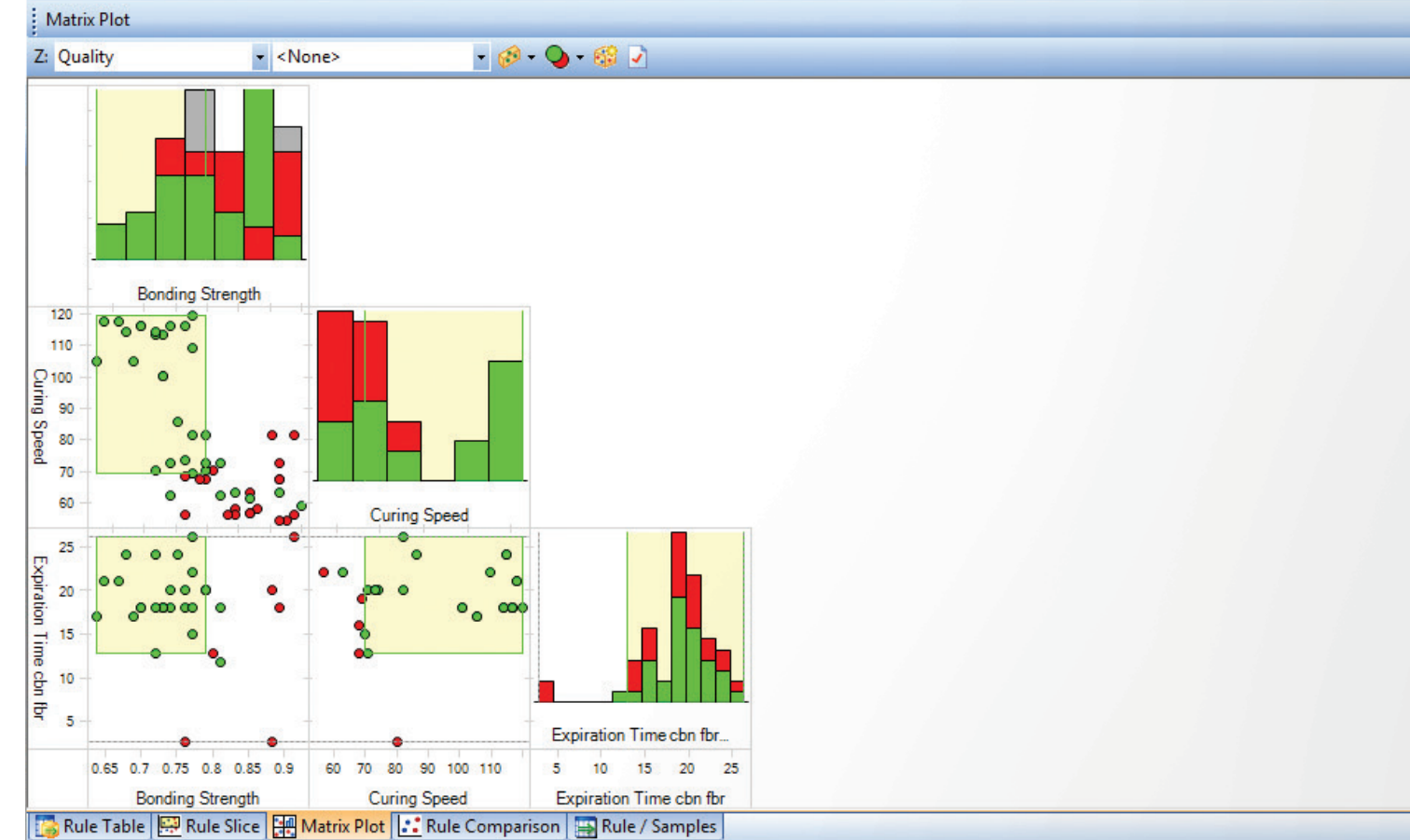
Visualization of Rules and Related Samples: A graphical view enables users to understand how samples are distributed within and outside of a rule.
