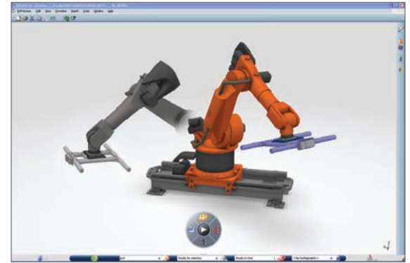
DELMIA Robot Task Definition enables the creation, programming, simulation and validation of the entire robot workcell.
