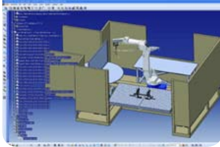
A DELMIA Robotics simulation for the design of welding fixtures.
