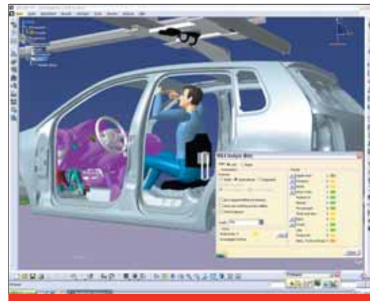
When manufacturing the latest Polo, the option of applying an installation seat was considered digitally – here when installing the sun visors
