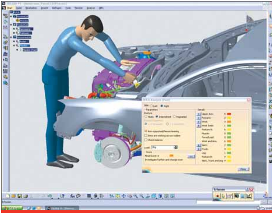
An additionally superimposed field of view enables a detailed view of the component that should be reached
