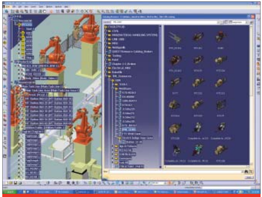
Body-in-White Workcell with Weldgun Library
