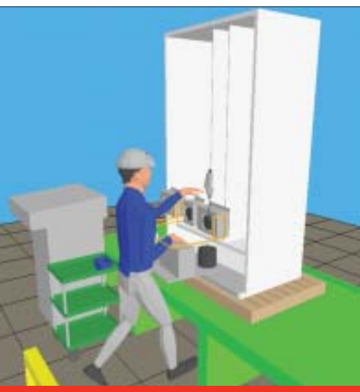
Fig. 2: Work verification by assembling digital mockups and conducting process simulations using digital manikins
