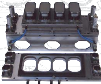
Fully automated thermoforming mold for production of lids.
