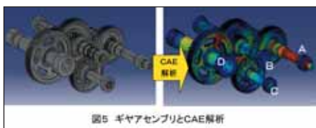
A gear assembly analysis performed by designers directly in the design environment.
