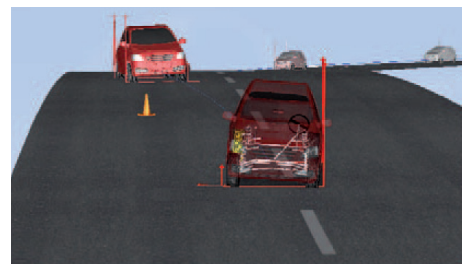
Vehicle on a segment-based road with a closed-loop driver testing the ability to avoid an obstacle hidden by a crest.
