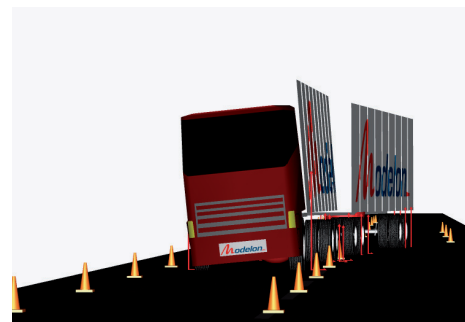
Truck-trailer combination with a closed loop driver model negotiating a double lane change.
