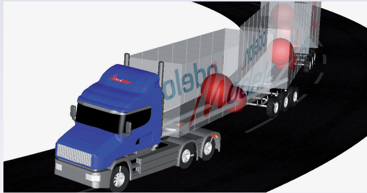
Road train configuration with three semi-trailers in curve stability test with closed loop driver model on 3D road.
