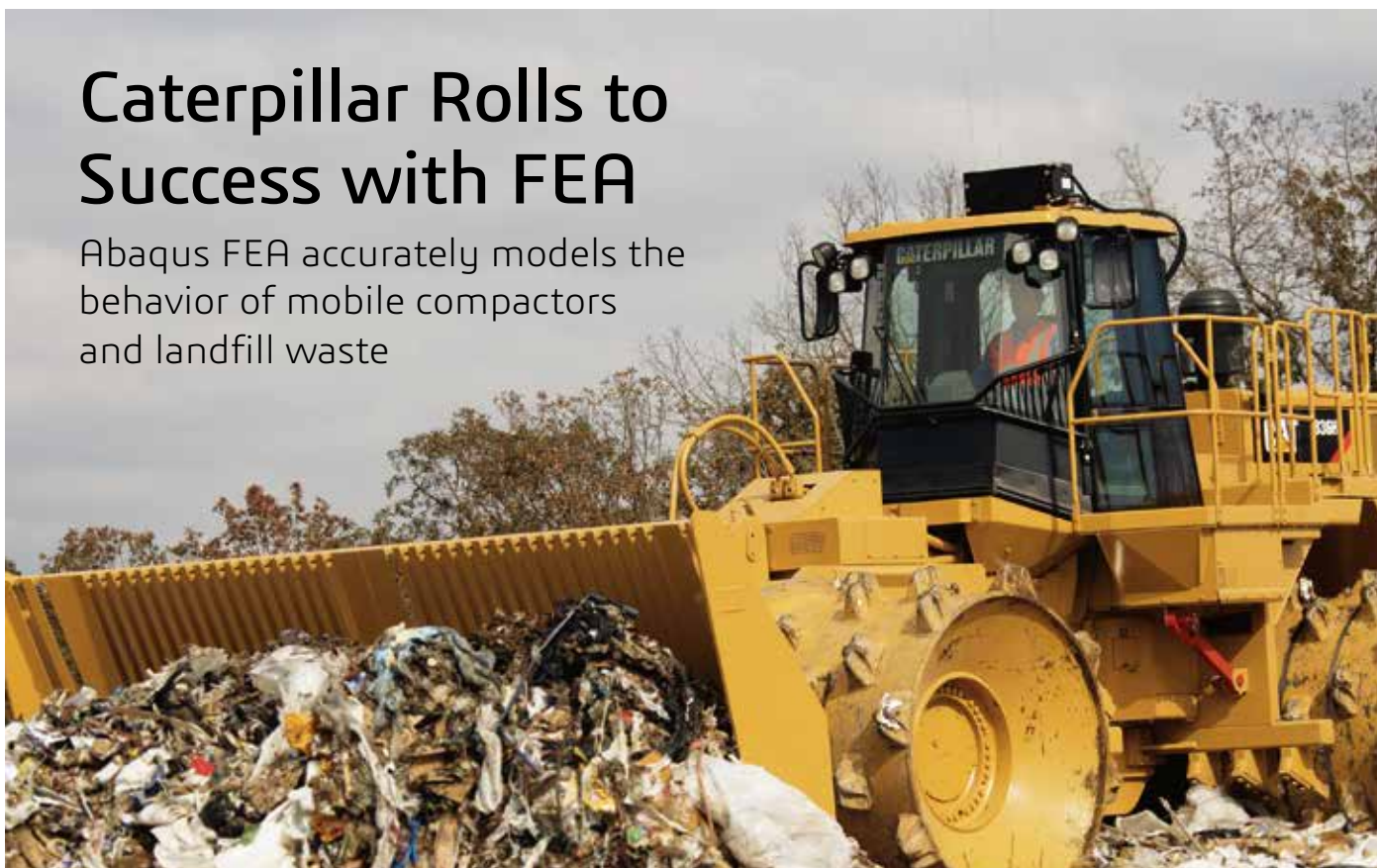
View of a Cat® landfill compactor, showing the patented drum tip technology that offers greater compaction and traction.
