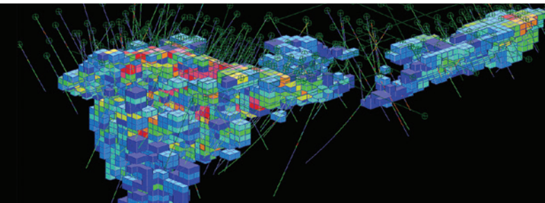
Block model constrained and coloured by grade with drill hole traces displayed.
