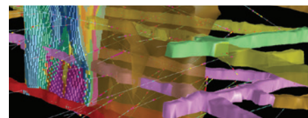
Surpac at a base metal operation. View drillholes, under-ground workings, ore zone and resource block model.
