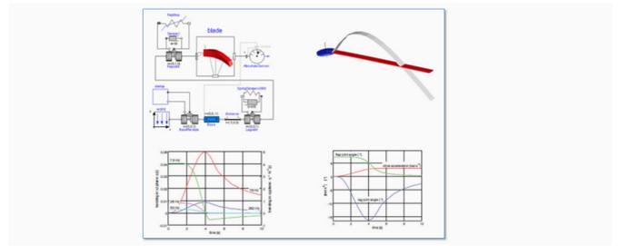
Simulation of a helicopter rotor blade system and the resultant blade deflection
