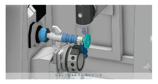
DELMIA, working with customers and tool manufacturers, has developed a very effective strategy called Adaptive Concentric Milling, which cuts hard material rapidly while prolonging the life of the tool.
