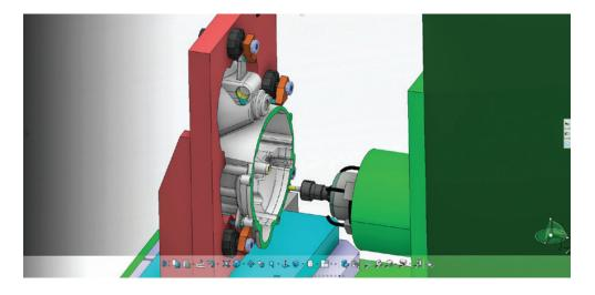
Four-head machines can be replaced with a mill-turn machine that uses DELMIA Machining with integrated simulation to generate both the toolpath and the rotation. No interaction is required, so the machine can be in production 24/7 and turn out superior quality—a major step forward in ROI.
