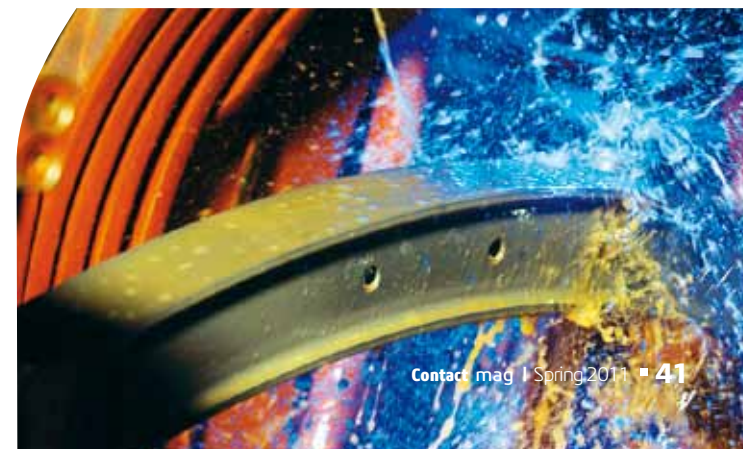
Slat track: Magnetic particle inspection of potential cracks
