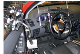
The test vehicle is equipped with car body levelling sensors, a steering robot, torque measuring wheels and a gyro platform.
