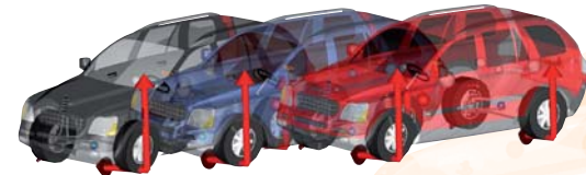
Example of responses (black, blue and red) for a vehicle with three different values of a perturbed parameter.
