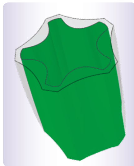
"Origami" concept vacuum panels are included in a PET container for designed collapse that compensates for shrinkage during cooling to maintain structural strength and integrity. Original shape is clear, final shape is green.
