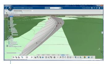
Changes in terrain preparation automatically translate to excavation preparation
