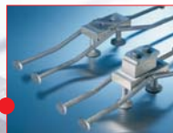
Peikko® PC corbel system is designed to support precast concrete beams and composite beams to reinforce concrete columns. The PC corbel also allows small variations of the corbel height at the construction site.
