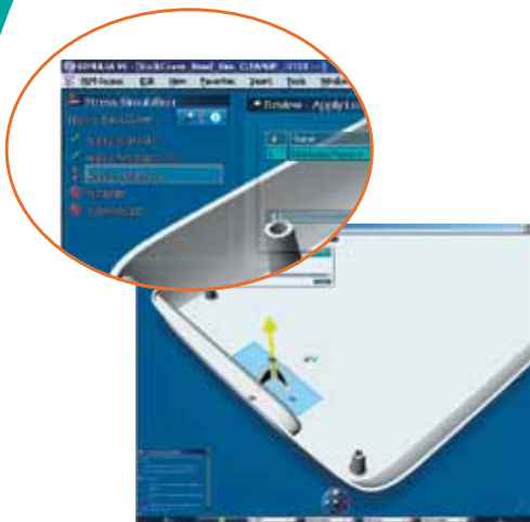
Loads: Define the load value according to the part's performance requirements, based on typical customer usage.
