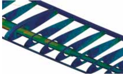
Figure 4. Traction loads applied directly to the main spar of the v-44 Albatross wing-sail.
