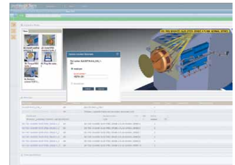
Digital Process Work Instruction Player is a delivery mechanism for DELMIA-authored 3D dynamic planning to the shop floor, tightly integrating execution, process control and data collection.
