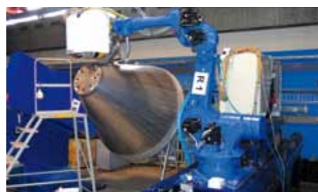
Robot inspects and welds sandwich cone structure.
